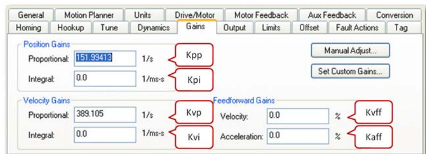
Figure 3 - Sercos Control Loop Gains in the Logix Designer Application
