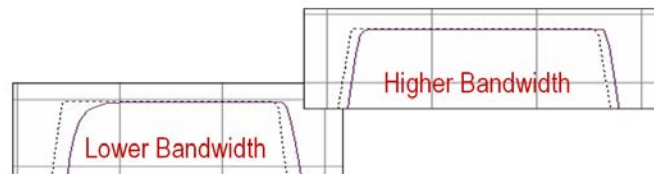
Figure 8 - How Bandwidth Affects Transient Response
